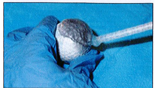
Top: The AccuTrans system. Bottom: In Figure 1, the investigator applies magnetic fingerprint powder to a golfball's surface before using AccuTrans.
